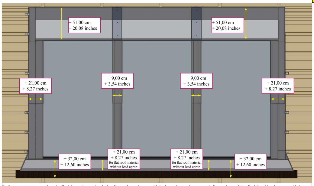
Before you start mounting the flashings please check the dimensions above, which show the ready mounted dimensions of the flashing. You have to add the dimensions of the flashing to the dimensions of the solar-panel so you will get the ready mounted dimension of the whole solar-system.
