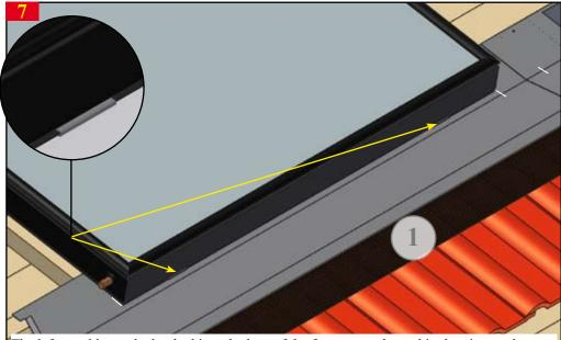
The left panel has to be hooked into the laps of the forepart as showed in the picture above. The panel must be moved until the left edge reaches the marked sign on the forepart.
