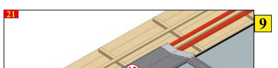
The mounting of the back-parts starts with the left one. You have to fit it in the left lateral-part and hook it into the upper edge of the panel. **Do not fix the back-part now.**
