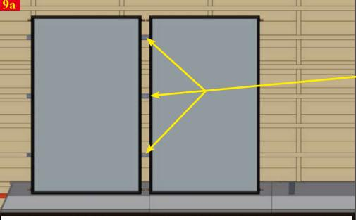
After you have placed the second panel, fix it with the longer fixation brackets together with the right side of the first panel. See the detailed picture on the right side. If you have only a 2-panel-system you can start fixing the right side of the second panel, in the same way as the left side of the first panel.
