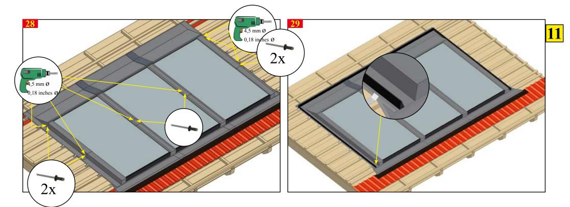
Fixation with rivets: You have to fix the single parts with rivets on the points shown in the picture. There are only holes in the covering parts so you have to drill that you can place the rivets.
