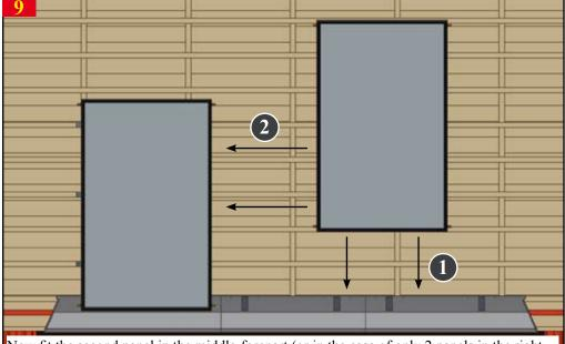
Now fit the second panel in the middle-forepart (or in the case of only 2 panels in the right forepart). The second panel must be fitted in the same way like the first one.
