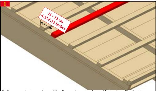
Before you start mounting of the foreparts must ad an additional roof batten to stabilisize the foreparts. The distance for this additional roof batten please see in the picture above.
